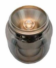
The Eimac Y-847A is a planar triode specifically designed for high voltage regulator or switch tube (pulse modulator) service. The compact, rugged design has very low internal inductance and capacitance to provide fast rise and fall times in pulse applications. The tube may be mounted in any position and is capable of enduring substantial vibration and shock.
